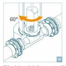
If the pig insert is in the correct position it can be turned. Turn insert by 60° as far as possible. Check by means of a tensile test if the insert is properly locked.
