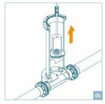
Remove pig insert from Quick Pig Station. Clean both pigging shaft and insert if required. Check insert for damages.
