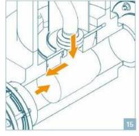
Now pump water into Quick Pig Station. The water flows behind the pig and fills the space between pig and valve. The generated pressure drives the pig through the pipeline.
