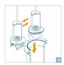
Important !! After the pigging process the receiver unit must be exchanged against the standard pig insert unit.
