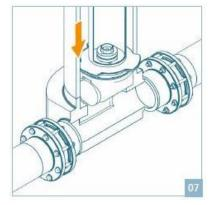
Reinstall pig insert into Quick Pig Station. The top of the pig must show into flow direction. Press down pig insert beyond gasket.
