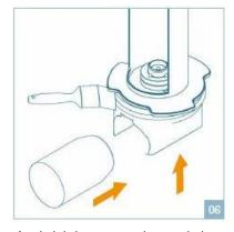
Apply lubricant to gasket at pig insert. Insert pig from the side or from the bottom.
