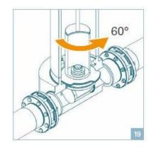
In order to remove the pig turn wrench by 60° counter-clockwise as far as possible.
