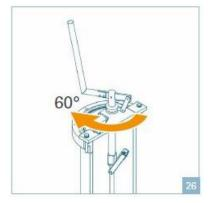
If the pig insert is in the correct position the lever can be turned clockwise by 60°. Then the pig insert or pig receiver unit is properly locked.
