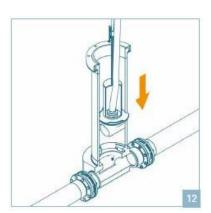
Apply lubricant to the gasket at pig insert as described in picture 6. Reinstall pig insert into Quick Pig Station.
