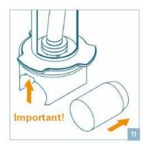
The opening of the insert must show opposite to the pig direction. During the pigging process the top of the pig must show into flow direction.
