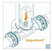
After pigging the blind cap must be mounted to the Storz coupling again.
