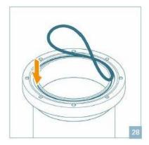
Reinstall O-ring gasket. Then screw flange cover to Quick Pig Station again.
