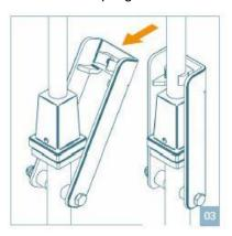
Apply underground hydrant wrench (DIN 3223C) and fix insert with locking device.
