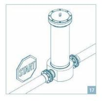
The pipeline can be pigged now. For this purpose pressurize pipeline again. You will notice at the insert steel rod system and from the sound when the pig has been caught.
