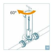
Press down pig receiver unti beyond gasket. Then turn insert 60° as far as possible.
