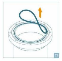
Before applying the lever remove the flange cover and the O-ring gasket.
