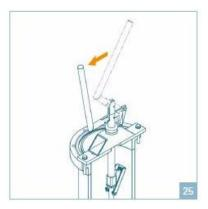
Move lever in such a way that the pig insert moves downward.
