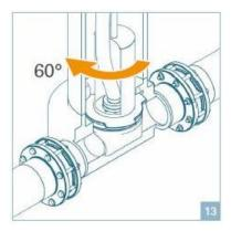
Press down pig insert beyond gasket. Then turn insert by 60° as far as possible.
