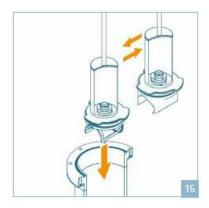
After having removed the pig insert install pig receiver unit into Quick Pig Station. The top of the pig-receiver unit must show into flow direction.
