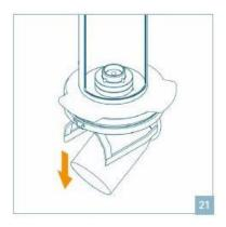
Check if the pig was received in the receiving basket. If not, repeat steps 15-20. Remove the received pig from the device.
