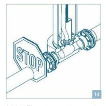
Advice: The valve must be opposite to pig direction and be closed.
