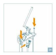
Apply lever to rectangular connection at pig insert respectively receiver unit. Fix lever to Quick Pig Station using screws of cover.
