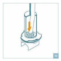
For flushing or pigging via Storz coupling remove blind cap. After this connect a suitable hose to the Storz coupling in the pig insert.
