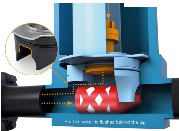
Possibility to launch from the Quick Pig station
