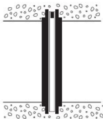
Placement of W802 in concrete floor and wall
